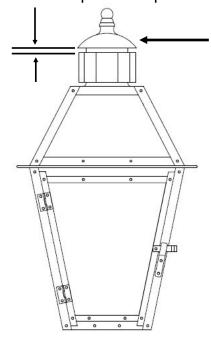
6. Slide the chimney cap and copper finial over the threaded nipple and secure in place with the brass ball nut.
