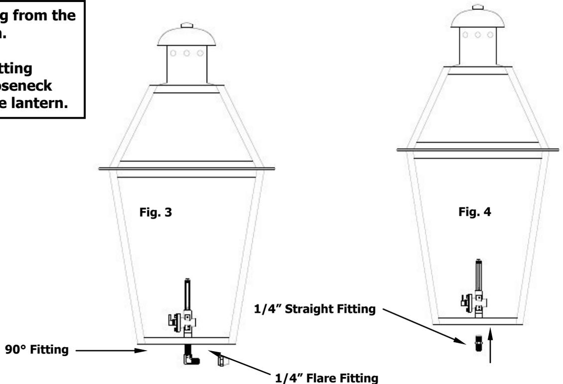
**6. Connect the gas line from the Gooseneck onto the Bottom of the lantern. Figure 5.**
