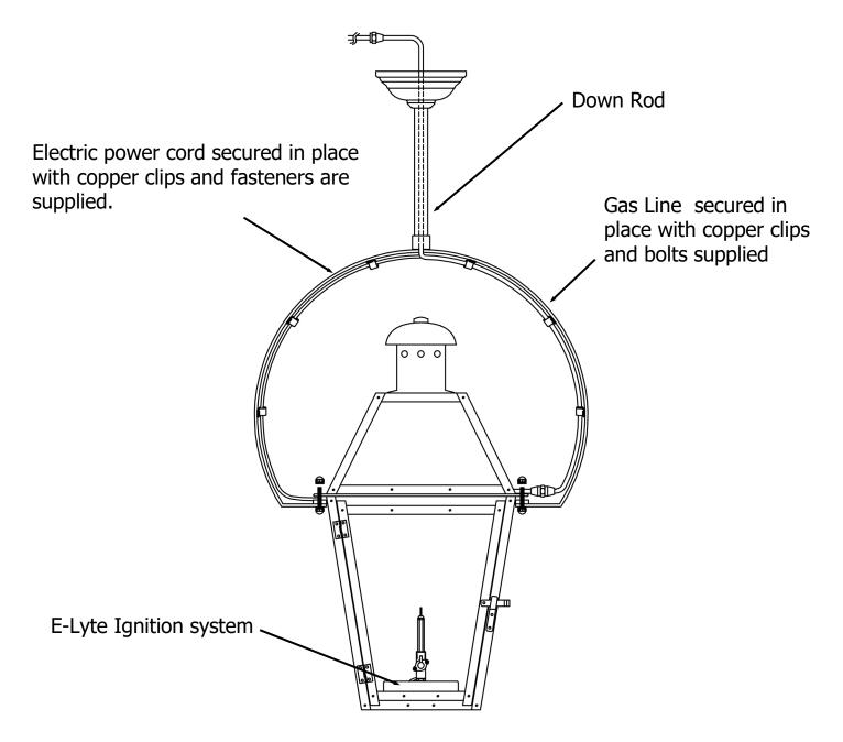
Lanterns that are equipped with an E-Lyte electronic ignition system are required to have a 120 Volt Ac power supply ran on the opposite side of the Yoke and up through the down rod. The securing clips and fasteners are supplied.
