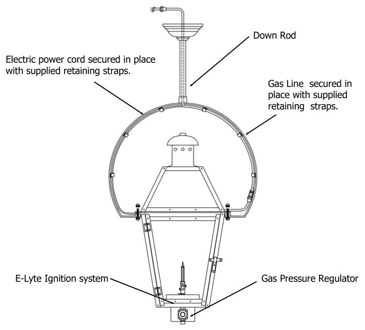
Lanterns that are equipped with an E-Lyte electronic ignition system are required to have a 120 Volt Ac power supply ran on the opposite side of the Yoke and up through the down rod. The securing clips and fasteners are supplied.
